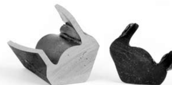
Aluminium casting with porosities. 1:1 reproduction on the impression. Material: Technovit Provil BLACK
