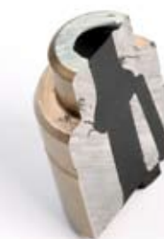
Longitudinal section through an injection nozzle. Impression of the canals with Technovit Provil BLACK.
