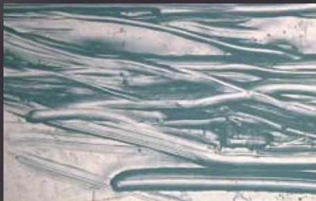
a 200x magnification of the impression with Technovit Provil
