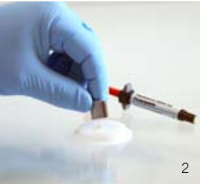
1 – Put Technovit fixing paste onto the bottom of the embedding form. 2 and 3 – Sample positioning 4 – Cure the fixing paste with the Technovit Blue LED; embed the sample as usual
